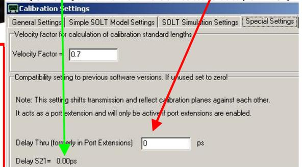
If using an empty Female Thru adaptor (no center conductor no PTFE insert) then the SMA male center conductor is used as the Open standard. Thus the delay used is very small being -12.8ps.
