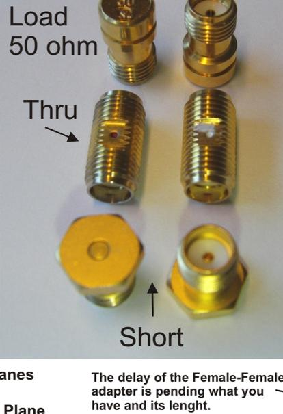
On this sheet you will find the settings required in "Calibration Settings" and "Simple SOLT" for the Reflection (S11/S22) and Transmission (S21/S12) calibrations.
