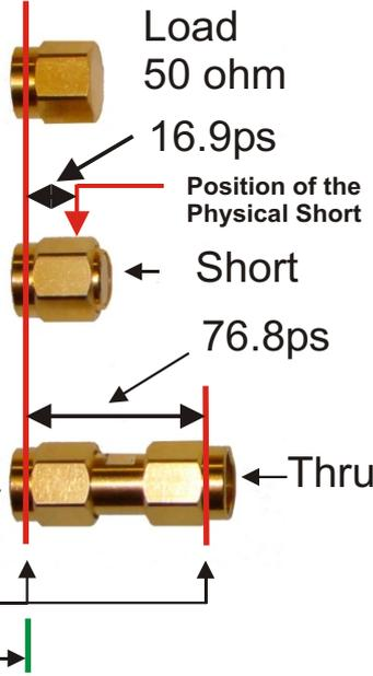
On this sheet you will find the settings required in "Calibration Settings" and "Simple SOLT" for the Reflection (S11/S22) and Transmission (S21/S12) calibrations.
